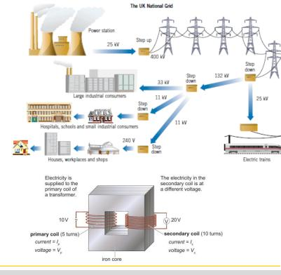
The national grid is a network of wires which deliver electricity safely from power stations. Step up transformer increase the voltage to reduce energy loss due to heat when moving large distances by transmission lines. Step down transformers decrease the voltage to safer levels.
